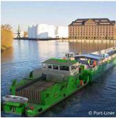
In 2020, the push boat Elektra will sail with green hydrogen and electric power from Berlin to Hamburg. The all-electric, hybrid propulsion is a project of the National Organisation for Hydrogen and Fuel Cell Energy (NOW) and supported by the German Ministry of Transport. The fuel cells are powered by green hydrogen from wind farms.
